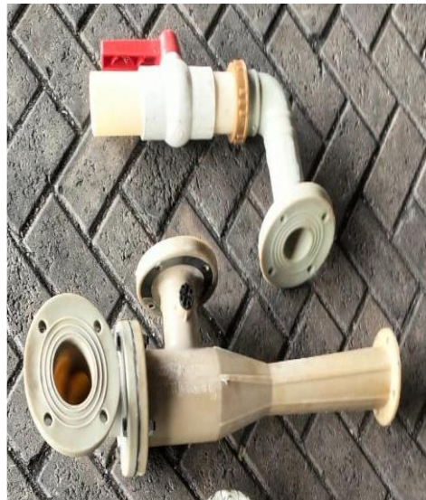
Gambar 7. Valve Parts dan Jet Device.
