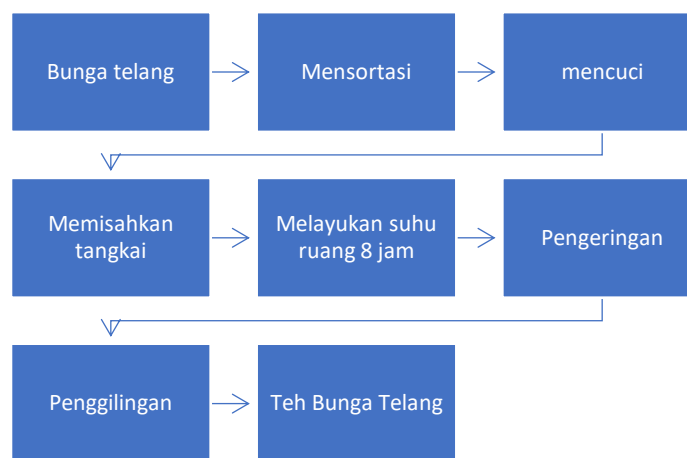
Gambar 3. Diagram Alir Proses Teh Bunga Telang
